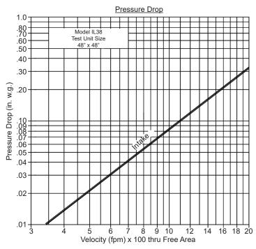
Intake air converted to standard air density.
